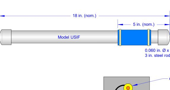
This sensor can also be used as the working electrode for a three electrode linear polarization test, or as one electrode for semi-quantitative resistivity measurements on soil between the electrode and structure.
