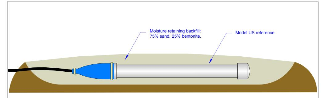
When installing a Model US reference electrode in a horizontal position, best performance will result if the electrode is placed in a small cavity in the soil. Once the electrode is positioned, cover it with at least an inch of a moisture retaining backfill. Thoroughly wet the backfill with potable water. Measure and record the potential using a recently calibrated portable reference electrode.
