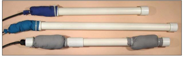
Reduced diameter underground reference electrodes were developed to simplify the installation of permanent underground electrodes in congested locations. They can be installed in a 5 cm (2 inch) diameter bore hole which makes them ideal for retrofit installations beneath paved surfaces. Since these electrodes weigh about one fifth as much as standard bagged electrodes, they are favored when product shipping costs are an important consideration.
