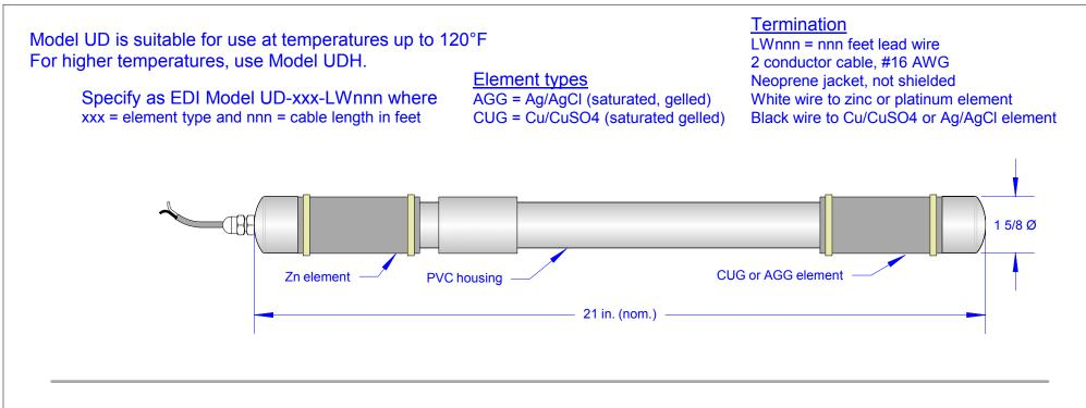
Model UDH is limited to a maximum service temperature of 200°F. When it is used beneath a storage tank containing heated product, it should be buried deep enough so that the temperature at the electrode is less than 200°F.
