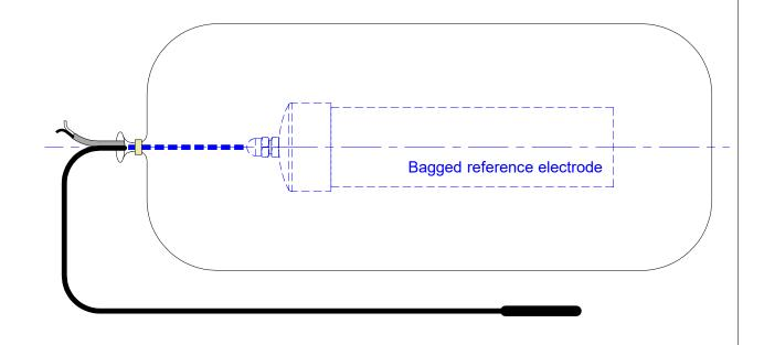
This sensor can also be used as the working electrode for a three electrode linear polarization test, or as one electrode for semi-quantitative resistivity measurements on soil between the electrode and structure.
