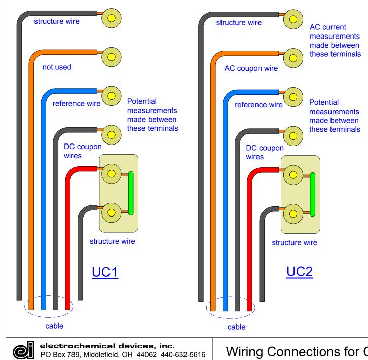
Wiring - Connect a structure wire and one of the DC coupon wires to a terminal pair that can be shunted through a switch or shorting bar. For convenience, a magnetic switch such as EDI Model UI-MS may be used. Connect the other DC coupon wire, the second structure wire, the AC coupon wire and the reference wire each to their own terminals.
