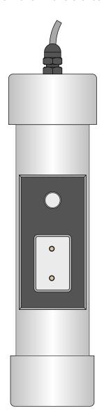
All coupons are internally connected to a 4-conductor 18 ga. cable. The red and black wires are connected to the DC coupon, the orange wire is connected to the AC coupon, the blue wire is connected to the optional zinc reference electrode.
