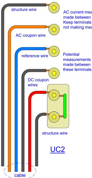
AC current measurements made between these terminals. Keep terminals shunted when not making measurements.
