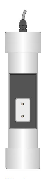
All coupons are internally connected to a 4-conductor 18 ga. cable. The red and black wires are connected to the DC coupon, the blue wire is connected to the optional zinc reference electrode, the orange wire is not connected on Model UC1. Specify as EDI Model UC1z-xxx-LWnnn where
