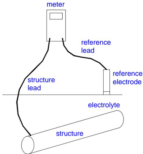
Figure 1a - Physical model of a potential measuring circuit.
