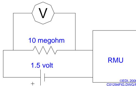
Figure 4 - Test setup for determining changes in input impedance of a data logger or RMU as it goes through its cycles. A 1 1/2 volt battery is connected to the input terminals through a 10 meg-ohm resistor. The voltage across this resistor is monitored with a portable voltmeter as the unit is put through its cycles. If the measured voltage exceeds 3/4 volts at any time, the unit may not be suitable for use with reference electrodes.
