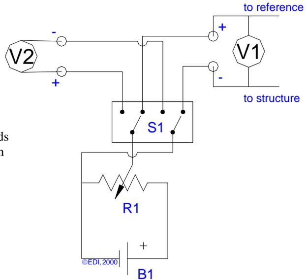
Figure 3 - Schematic of two meter potentiometric voltmeter converter. Adjust potentiometer until meter V1 reads zero. Change switch to opposite position to read potential. Potential shown on meter V2 will have the same sign of the actual potential.
