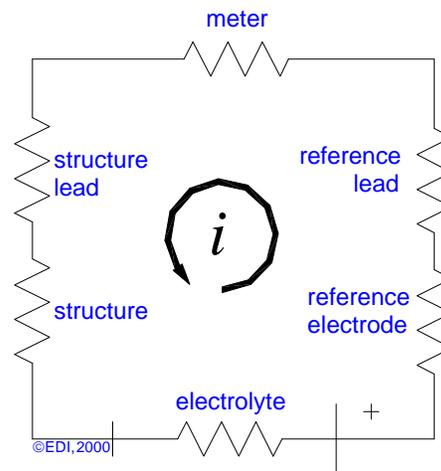
Figure 1b - Electrical model of a potential measuring circuit. The potential difference between the reference electrode and the structure is the driving force for the current flowing in the circuit.
